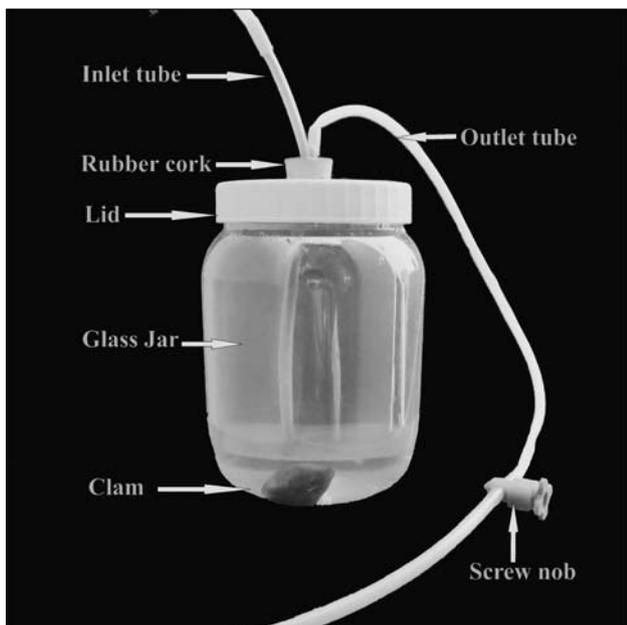
Fig.1 Respiratory apparatus used during experiments
